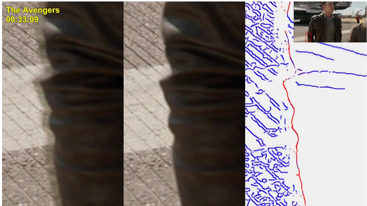
Figure 9: Example of edge-sharpness mismatch detected in The Avengers .
